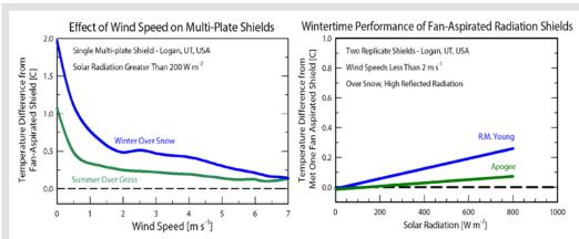
Left: Naturally-aspirated shields are subject to significant measurement errors when wind speeds are less than 3 m s $^{-1}$ . Errors increase when snow covers ground surface. Right: The performance of Apogee (model TS-100) and R.M. Young (model 43502) fan-aspirated shields relative to a Met One (model 076B) fan-aspirated shield.
