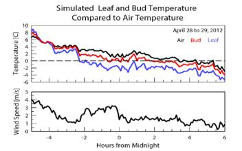
Above: Leaf and bud temperature approximations measured with an Apogee SF-110 compared to air temperature (top panel) and wind speed (bottom panel) on the evening of April 28, 2012. Leaf and bud temperatures were both below air temperature after 8 P.M. and reached freezing 6 (leaf) and 4 (bud) hours before the air temperature.
