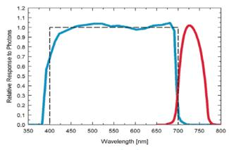
Spectral response of PAR detector (blue) and Far-red detector (red) compared to defined response of plants to radiation (dashed).
