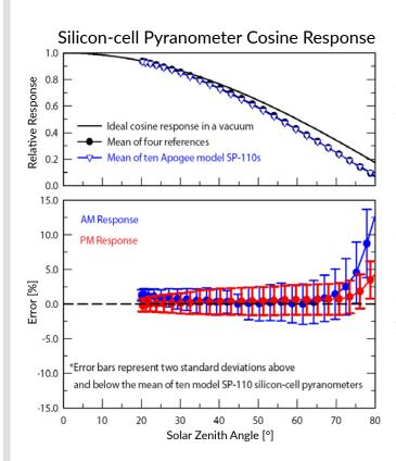
Top: Mean relative response of ten Apogee model SP-110 pyranometers and mean relative response of four reference pyranometers (Kipp & Zonen models CM11, CMP11, CM21; Hukseflux model SR20) compared to ideal angular (cosine) response in a vacuum. Differences from the ideal response are caused by atmospheric attenuation of solar radiation, which increases as solar zenith angle increases.
